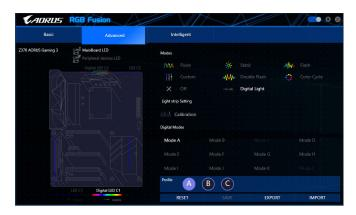
Advanced (Note): Allows you to configure the lighting behaviour and color of the LEDs in each region. You can
