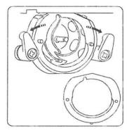
Open the hook race ring holders and remove the hook race ring.
