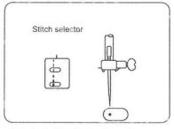
Use Left Needle Position for more. control while topstitching or edge stitching difficult fabrics.
