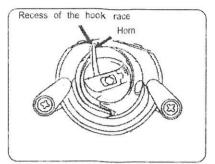
When inserting the bobbin case, place the horn into the recess of the hook race.
