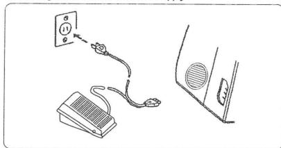
Before connecting the power, make sure the voltage and frequency of your electrical power conform to the machine.
