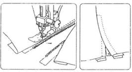
Pin or baste zipper tape to fabric and place it under the foot.
