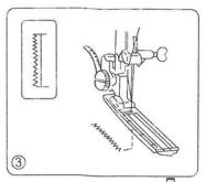
Set the stitch selector at " [ " , sew 5 stitches of bartack and raise the needle up from the fabric.
