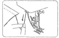
The threads are cut the proper length for starting the next seam.
