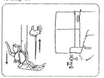
Turn the balance wheel toward you to raise the needle to its highest position. Raise the presser foot.
