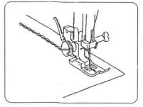
The stitch is sewn with two stitches forward and one stitch backward forming a seam that does not rip easily.
