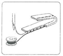
The needle thread and the bobbin thread should interlock in the center of two layers of fabric in straight stitch seams.
