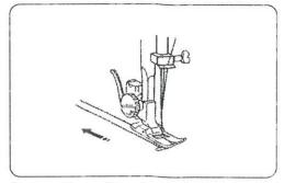
Pull 15 cm (6") of both threads back and under the presser foot.
