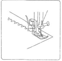
When forward and reverse feeds become unbalenced depending upon the type of fabric, correct the balance by turning the stitch length control as follows:
