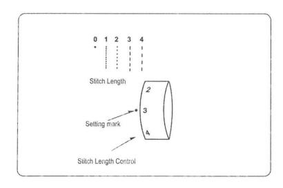
The sitch length control regulates the length of stitch, and also has a stretch stitches setting.
