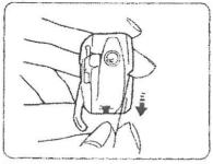
Pull the thread into the bobbin case slot.
