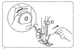
Turn the balance wheel slowly towards you with your right hand until the needle goes down and continue turning balance wheel until the take-up lever is at its highest position. Lightly draw up the needle thread forming a loop of the bobbin thread.
