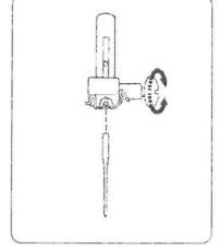
Undo the needle clamp screw just enough to release the needle.
