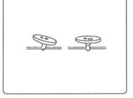
To strengthen the shank, cut the threads leaving a 20 cm (8") tail. Bring the needle thread down through the hole in the button and wind it around the shank.
