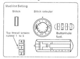
Make a test buttonhole and a sample duplicating the fabric, interfacing and seams of the actual garment . Place the button on the fabric sample and mark the top and bottom to determine the buttonhole length.
