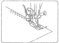
This type of stitch is used on the seam allowance to prevent fabrics from fraying at raw edges.
