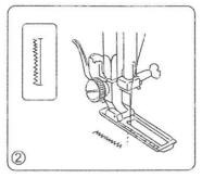
Sew down the left side stopping at the bottom mark. Raise the needle.
