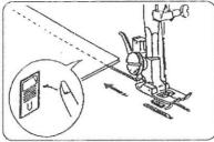
For fastening the ends of seams, press the reverse stitch control several reverse stitches.
