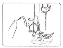
Press the lever on the back of the foot holder.
