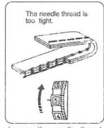
Loosen the needle thread tension by moving the dial to a lower number.
