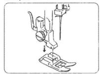
Place the presser foot so the pin on the foot lies just under the groove of the foot holder. Lower the foot holder to lock the foot in place.
