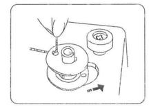
Draw thread from spool. Guide the thread around the bobbin winder thread guide.
