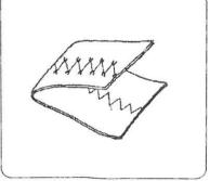
To obtain better zigzag stitches, the upper tension should be slightly lower than in the case of straight sewing. The upper thread should appear slightly on the reverse side of the fabric.
