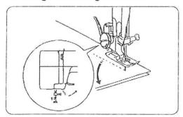
Stop the machine and turn the balance wheel toward you to bring the needle down into the fabric.
