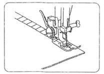
Overedge stitch will be done most successfully when the right side stitches of zigzag fall slightly off the edges of the fabrics.
