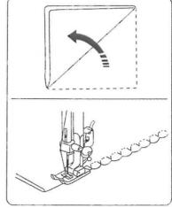
Place the folded edge along the slot of foot. The needle should fall off the edge of the fabric. on the right forming a tuck.
